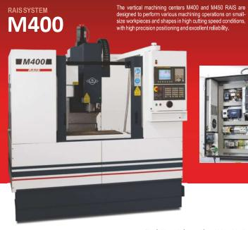
Optimum construction; minimum heat deformation; absence of vibrations in working process; high geometry accuracy.
