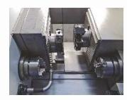
All structural parts are manufactured from high quality Meehanite cast iron and stress relieved for deformation.
