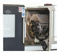
All structural parts are manufactured from high quality Meehanite cast iron and stress relieved for deformation.
